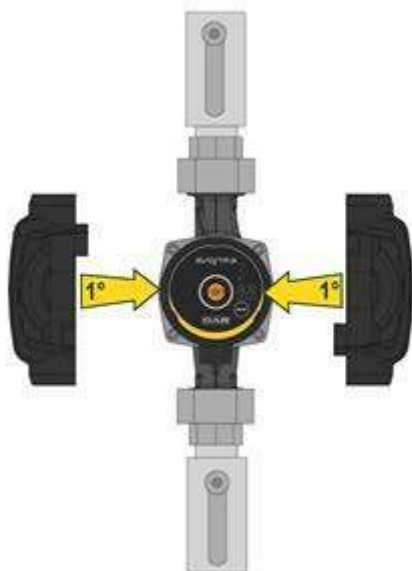
Figure 7: Insulating the pump body
