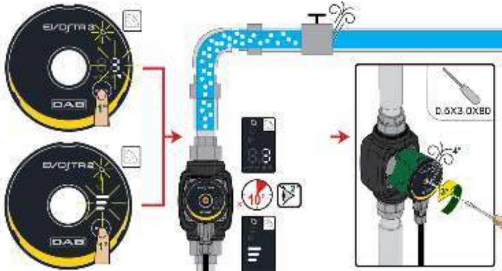
Figure 8: Venting of the pump
